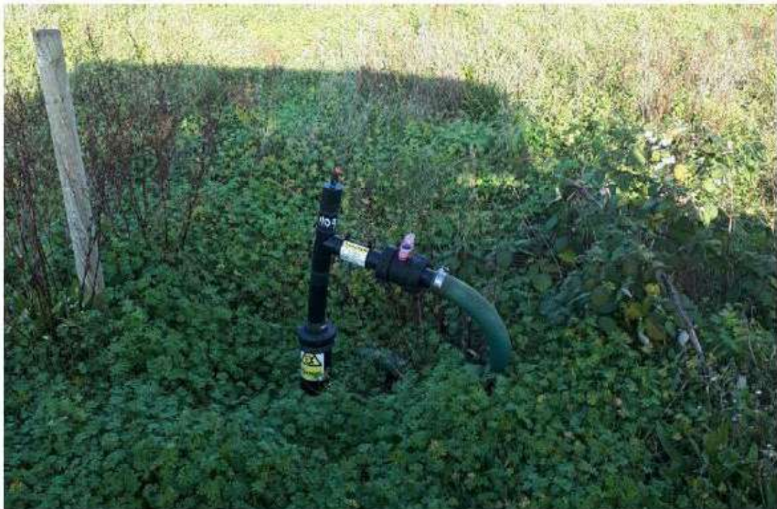
Figure 11: Close up of gas monitoring apparatus present within the application site.
